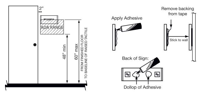
IMPORTANT: Prior to installation, remove all contents from box and inspect each sign for damage. Box should contain signs, hardware, and mounting instructions for each style of mount used. Surface of the sign must be handled with care. Clean with water and mild detergent.
