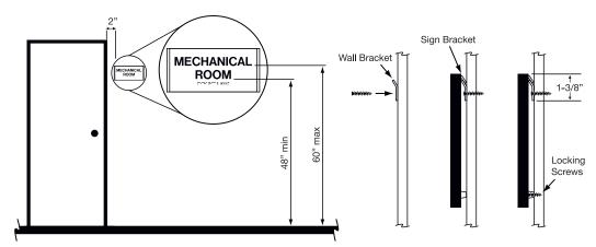
IMPORTANT: Prior to installation, remove all contents from box and inspect each sign for damage. Box should contain signs, hardware, and mounting instructions for each style of mount used. Surface of the sign must be handled with care. Bumpers are needed for proper function of end cap. Do not remove. Clean with water and mild detergent.
